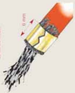
■ Fixing of screening to screened leads.
