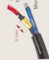
■ Coaxial cable: Fixing of screening to screened leads
