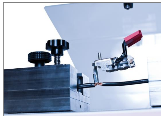
Universal clamping jaws for different sizes of crimps
