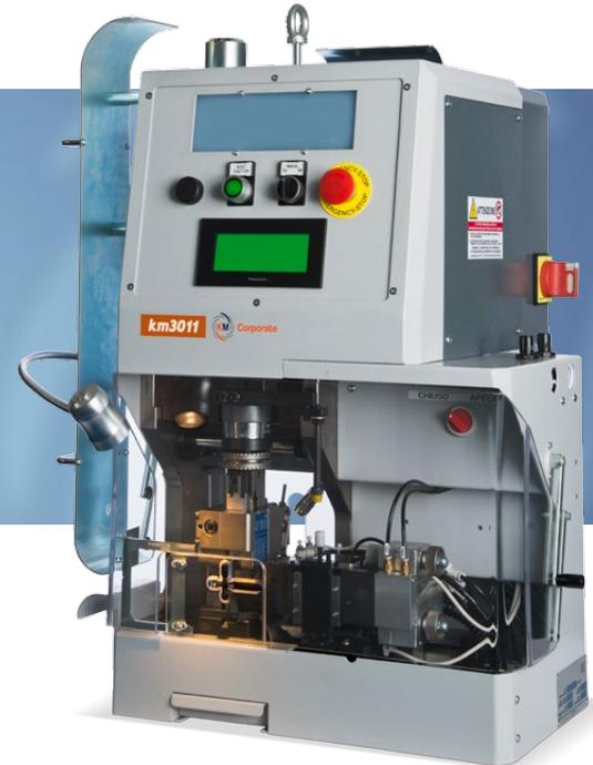
Model **KM3011** is an "IN LINE" stripper crimper so stripping and crimping operations are made without moving the wire so to guarantee a high stability of the process.
