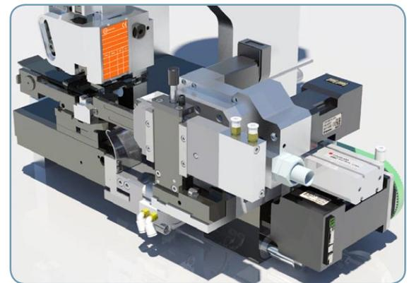
Model **KM3012** is the electronic version of the product range stripper crimper for performing stripping and crimping operations, but with completely programmable and actuated settings.
